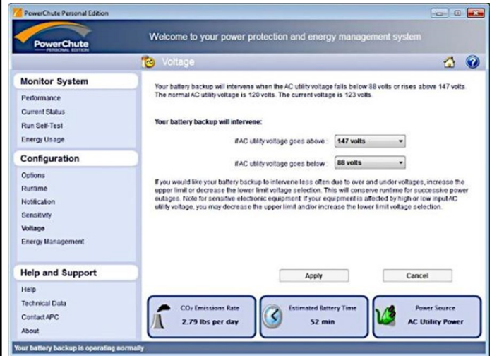
Figure 6. UPS Voltage Settings
